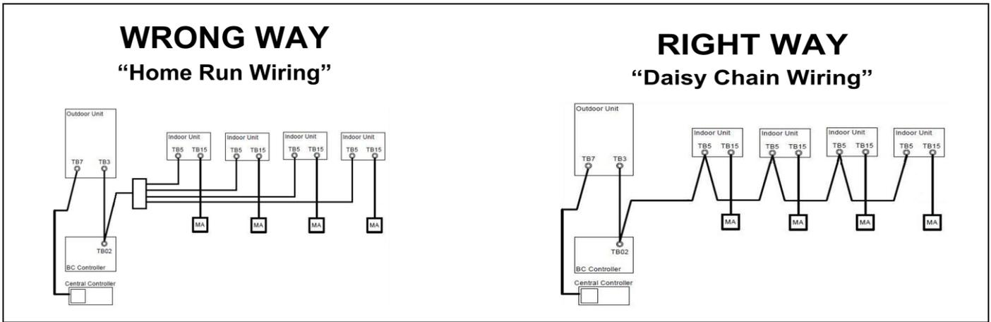
**18/2AWG stranded shielded cable** can be used if total control wire length is less than 656 ft. (Remember 16/2AWG stranded shielded cable is the recommendation for M-Net wiring). If this length is exceeded with 18/2AWG wire there may be a problem with the communications network and a 6607 ACK Error fault code may be displayed.
