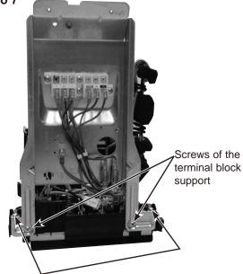
Screws of the ground wires and the terminal block support
