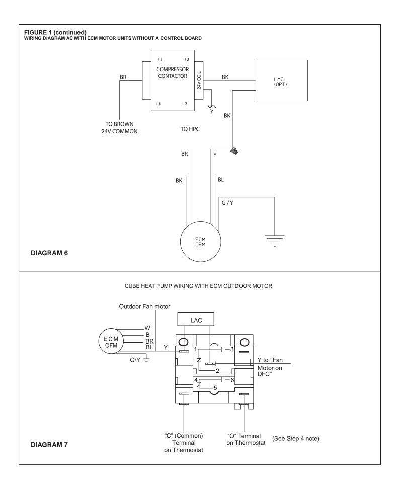
For Rectangle HP With ECM Motor: The outdoor fan motor blue lead is to be broken with the motor side going to the low ambient relay terminal 1 and the JEZ control side going to the low ambient relay terminal 2.
