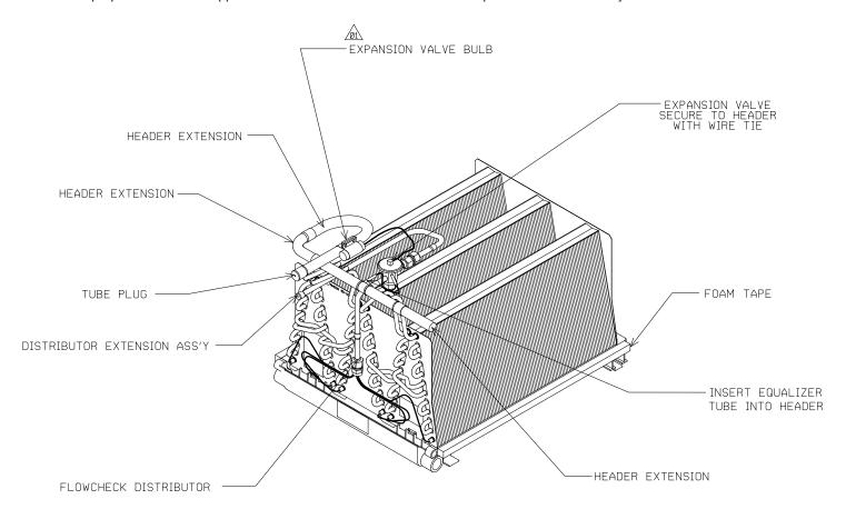
FIGURE 1. FRONT CONNECTION COIL
