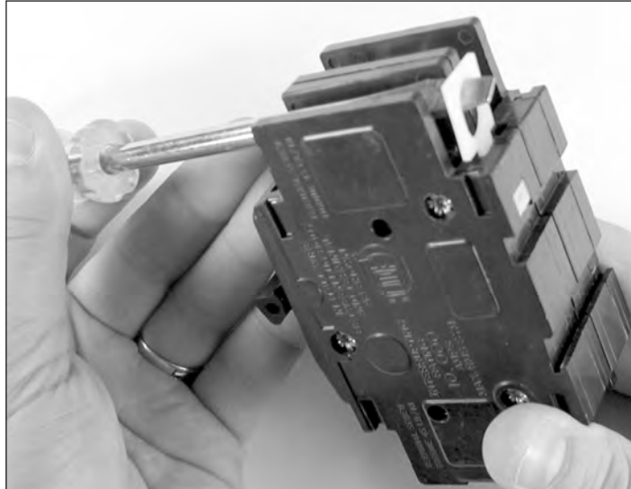
FIGURE 5 ROTATING CIRCUIT BREAKER
