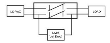
Load example: 600 Watt heater (600 W = 600 VA - 120V x 5A)
