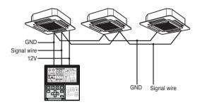
When controlling multiple indoor units with event communication function with one remote controller, you must change the master/slave setting from the indoor unit.
