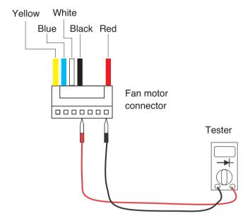
Check the PCB during the Power on
