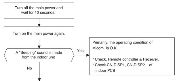
Check the voltage of power supply (AC220V/AC240V, 50Hz) and check for the following :
