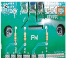
IPM : Measuring resistance between No.24,25 pin
