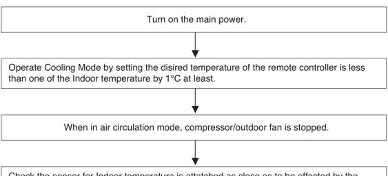
Check the sensor for Indoor temperature is attatched as close as to be effected by the themperature of Heat Exchange (EVA.)
