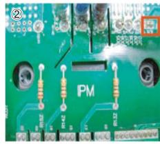
IPM : Measuring resistance between No.24,25 pin
