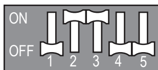
Figure 128: LMU180HV~240HV, LMU30-36CHV Night Quiet Mode DIP Switch Settings.
